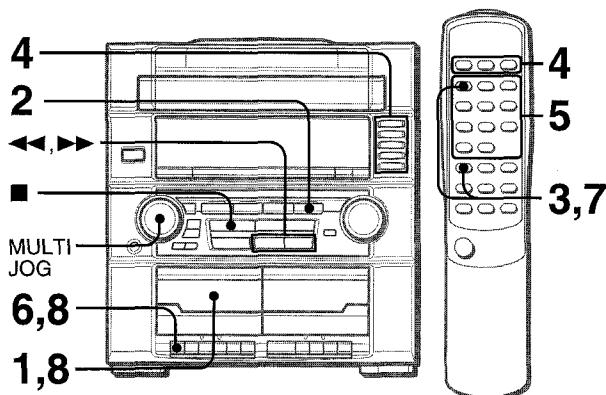
The AI edit recording function enables CD recording without worrying about tape length and track length. When a CD is inserted, the unit automatically calculates the total track length. If necessary, the order of tracks is rearranged so that no track is cut short.
